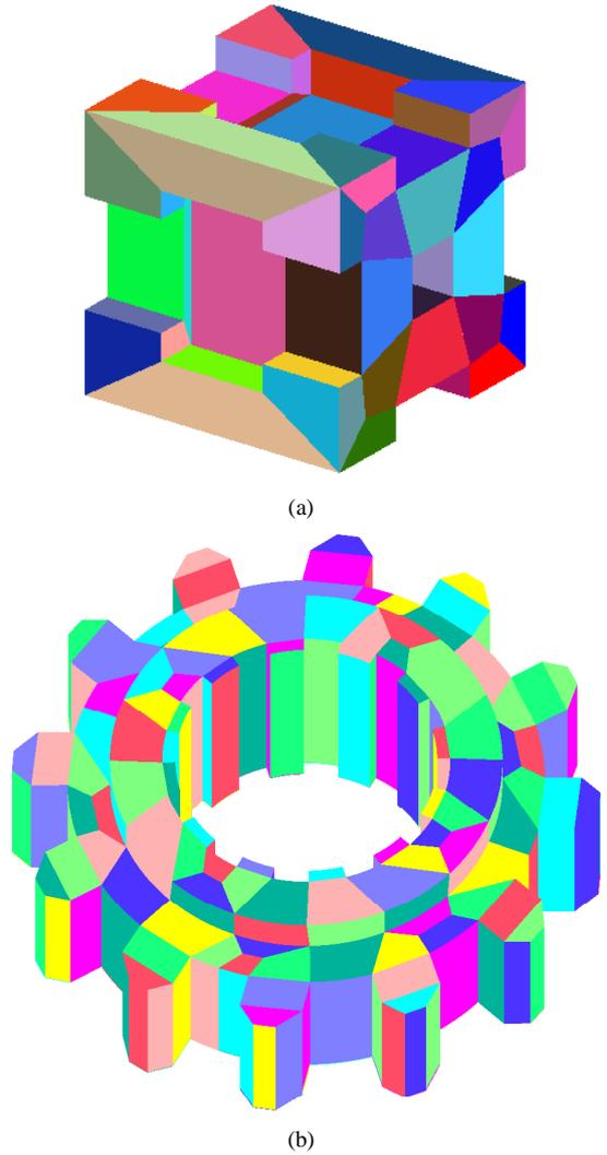
Fig. 12. Segmentation of CAD surfaces
